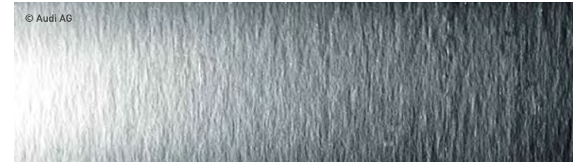
Laboratory sample with pronounced roping after cathodic electrodeposition.
